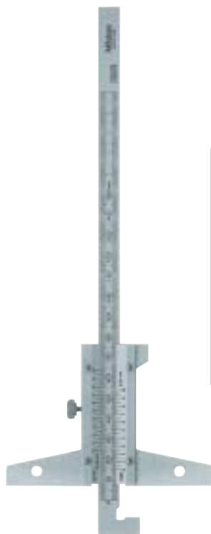
Reading on hook vernier and depth vernier
