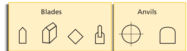
Various designs of knives and anvils for rotary cutting
