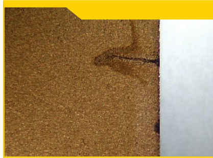
Standard Tungsten Carbide Standard tungsten carbide materials had multiple cracks on both rough and trim/finish cuts.
